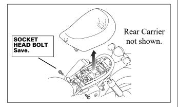
2. Remove two cap nuts, two large washers, and two 8 mm flange bolts (as shown).
