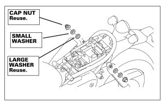
2. Reinstall the seat in the reverse order of removal.
