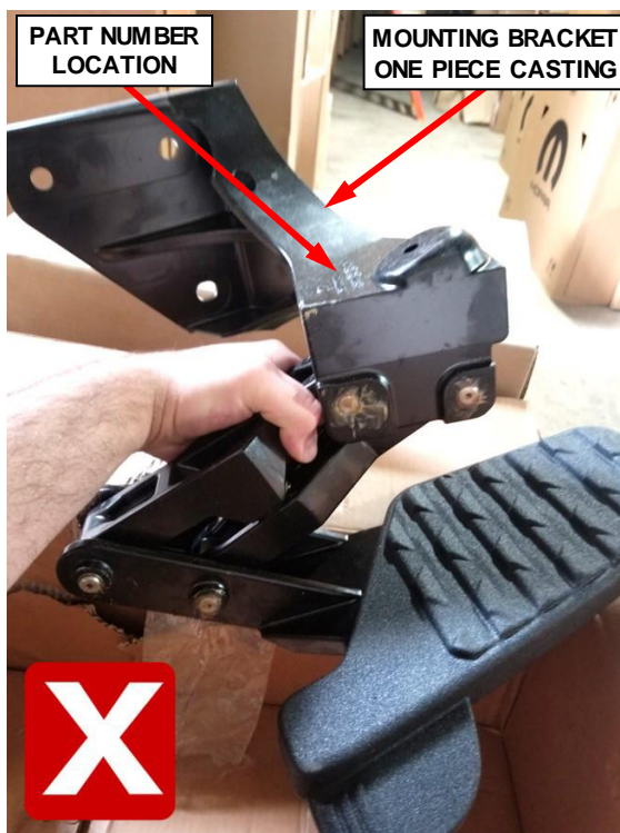
One Piece Casting Recalled Design Must Be Replaced
