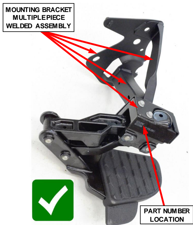
Multiple Piece Welded Assembly Current Design OK Do Not Replace
