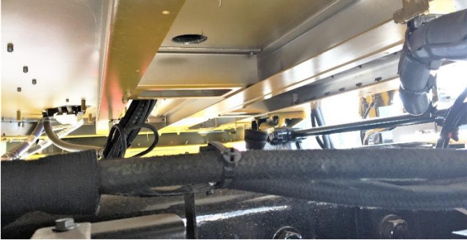
Figure 5. Inspect underside of cab before drilling
