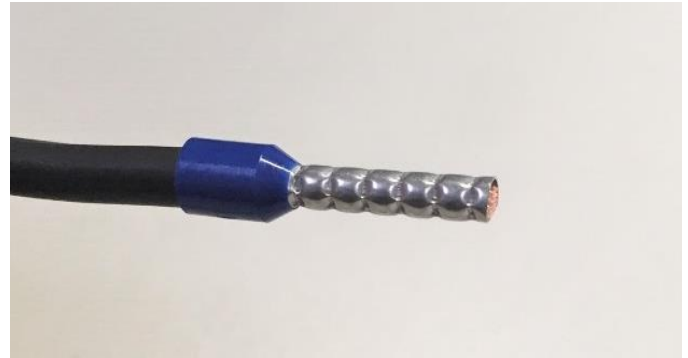
Figure 16. Ferrule crimp detail
