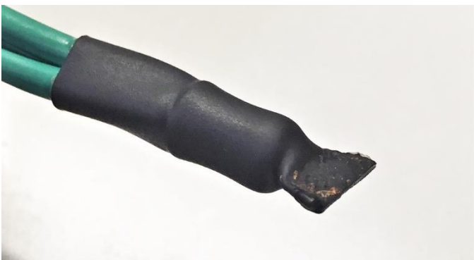
Figure 15. Completed ground crimp
