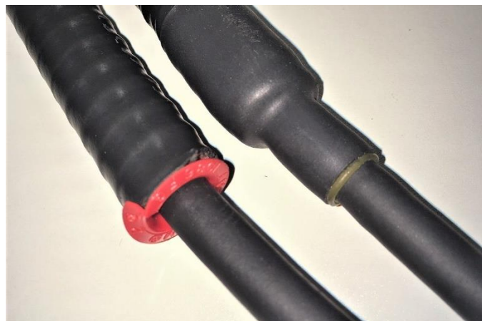
Figure 10. Anti-short bushing and heat shrink tubing installation detail
