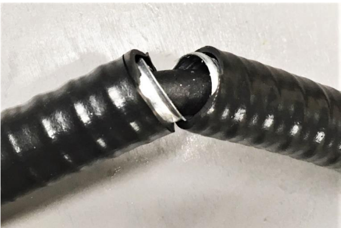
Figure 6. Conduit sheath separated
