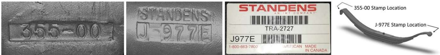
Figure 1 Showing Part Number (355-00) and Lot Number (J977E) physically stamped into the ends of each leaf spring. The part may also have a temporary label with Alternate Part Number (TRA-2727).
