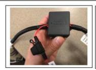
This Relay/Capacitor Harness Module (13" long) was installed under the Driver's Seat (Sprinters)
