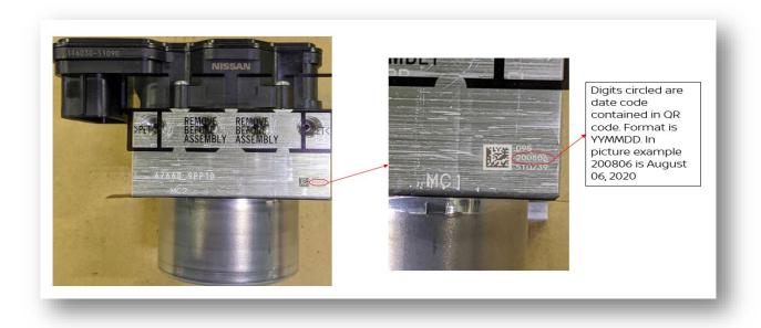
Alternatively, if the date code is damaged or illegible, a QR Code Reader application may be downloaded to a smartphone and used to scan the QR code to identify the manufacture date of the part.
