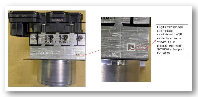
Alternatively, if the date code is damaged or illegible, a QR Code Reader application may be downloaded to a smartphone and used to scan the QR code to identify the manufacture date of the part.
