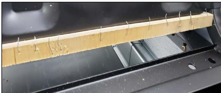
Figure 3: Remove Staples from Wood Strip
