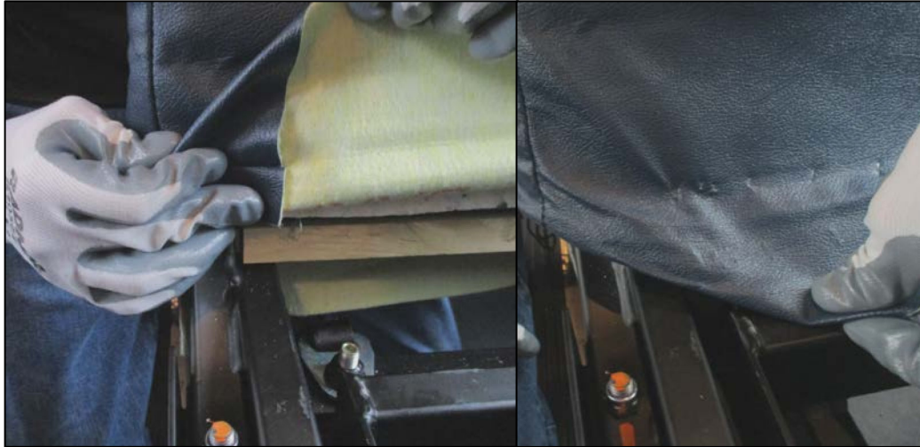
Figure 10: Folding and Tucking the Vinyl Seat Cover
