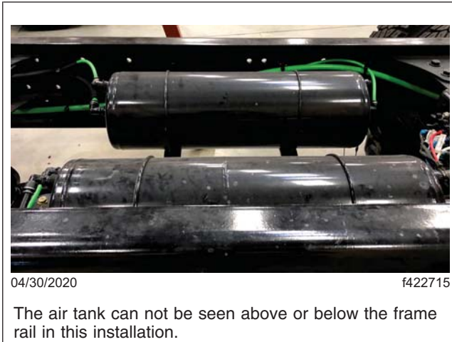
Fig. 1, In-Rail Air Tank, Top View
