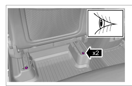
Make sure that the rear flange nuts are installed on both front seats.
