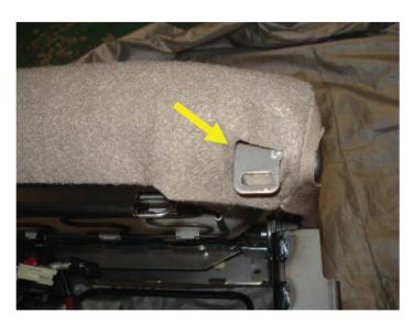
3. Secure all four retaining strips of the seat bottom fabric/leather to the seat frame.
