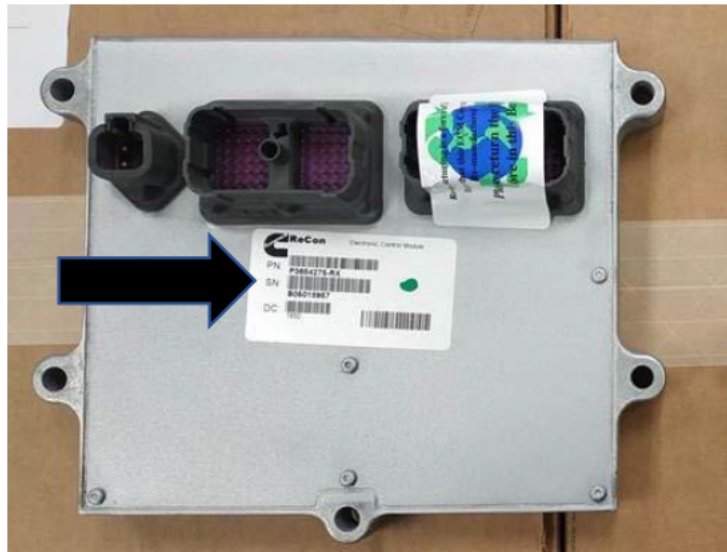
Figure 1 - Location of ECM Serial Number
