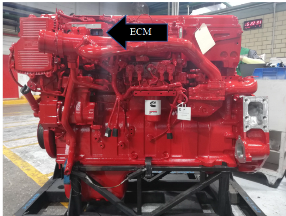
Figure 3 – Location of ECM on Engine
