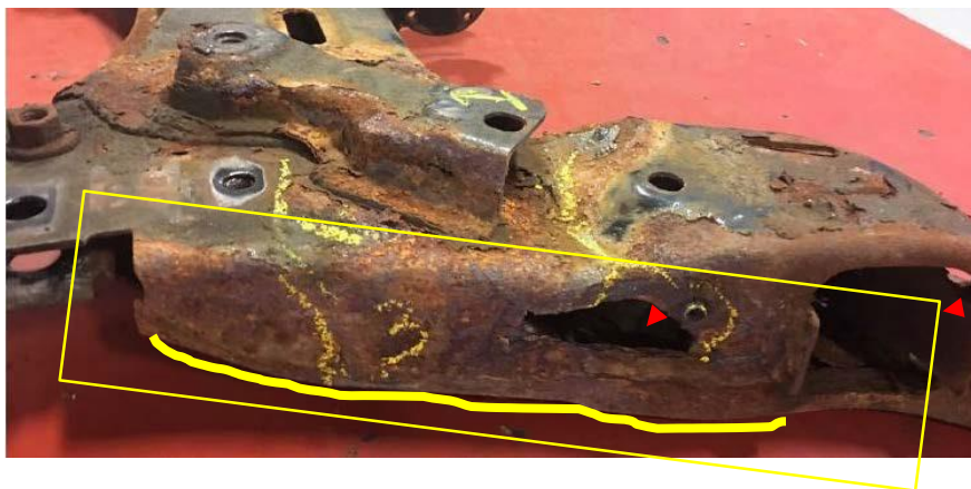
Top Side View: Damaged Cross member
