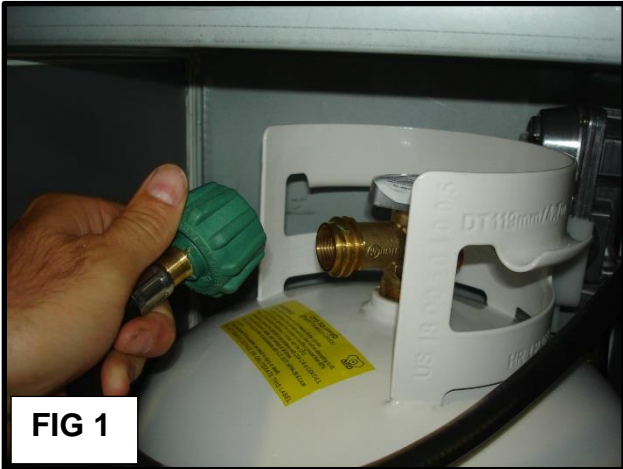
Fig 1: Turn off LP at tank. Disconnect the LP hose from the tank. Unfasten the tank strap/s, and remove the tank from the compartment. Fig 2: Replace each strap with a new one from the Recall Parts Kit.
