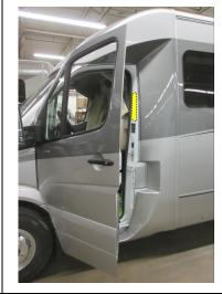
Remove the wax paper and apply the new self-adhesive yellow OCCC decal on the inside top of each cab door pillar with a squeegee.
