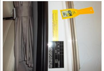
Use a solvent or similar adhesive remover with a plastic putty knife to scrape the decal off of the cab door pillar.
