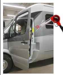
Open the driver door and locate the yellow OCCC decal (near head) rest. Warm the decal with a hair dryer or heat gun.
