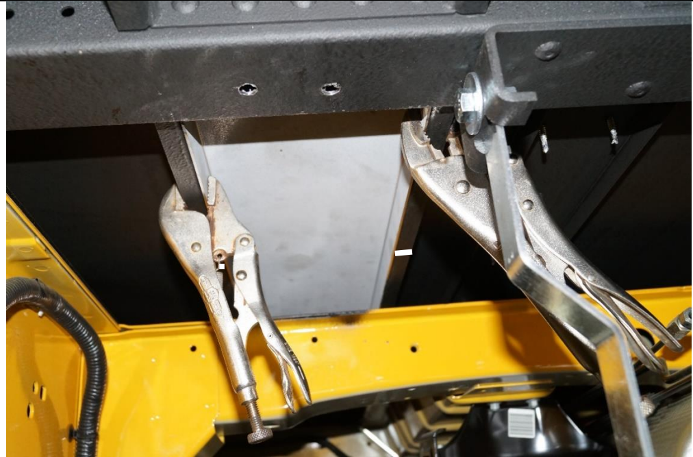
Figure 10 - Fixing the seat reinforcement
