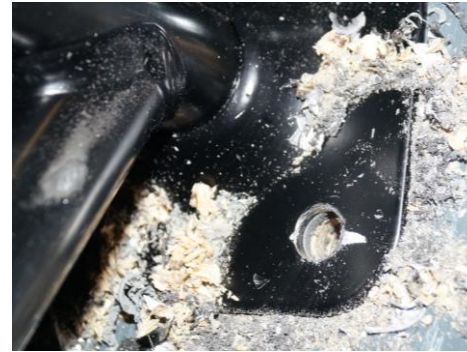
Figure 12 - Drilling from inside de vehicle
