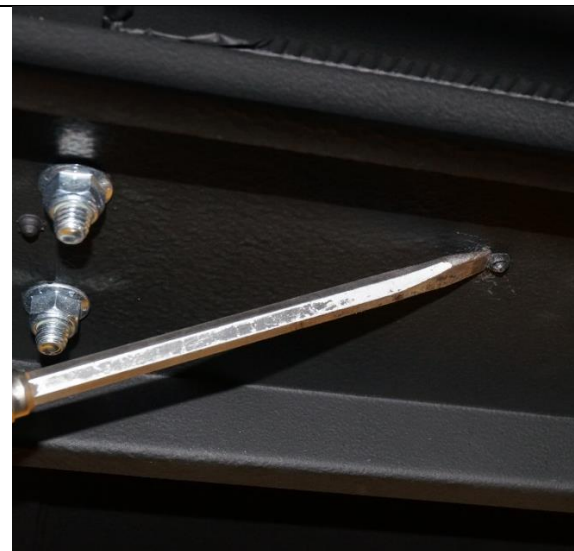
Figure 7 - Cutting rivet with chisel
