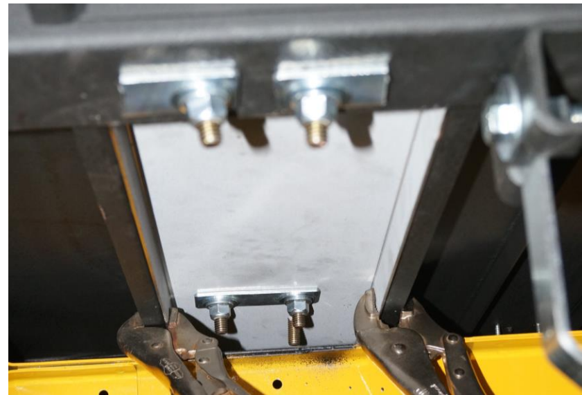
Figure 16 - Fixing the seat leg (under the vehicle)
