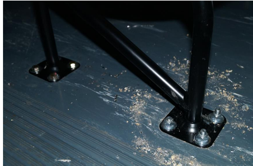
Figure 15 - Fixing the seat leg (in the vehicle)
