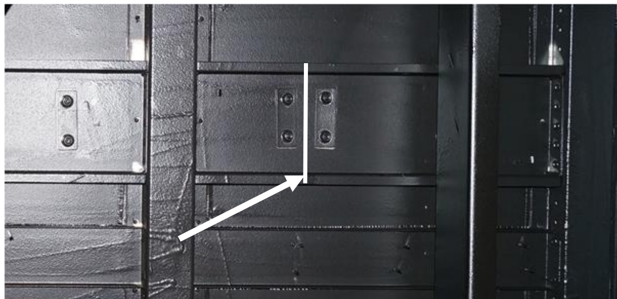
Figure 9 - Marking the center of the seat rear bolt pattern
