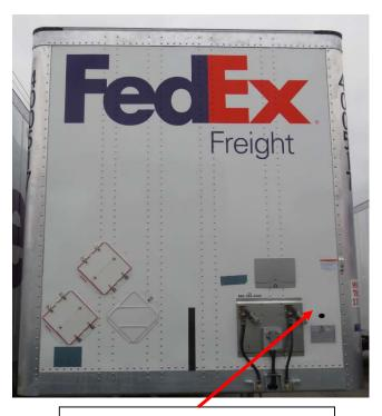
Notice the black paint dot above the VIN tag indicating that the repair has already been completed. If the black dot is not present it will need to be added once the repair has been completed.
