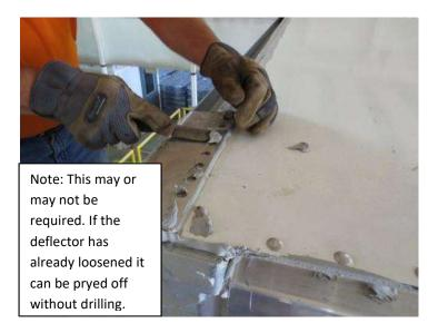
3. Using a 3/16" drill bit, drill out and remove the 4 existing rivets.
