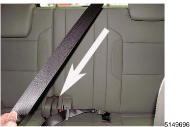
3. Pull the complete length of the seatbelt out until it reaches a hard stop.
