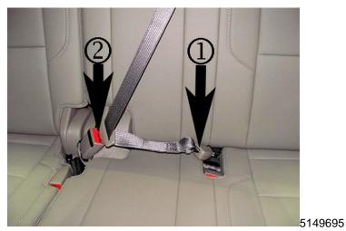
2. Pull the seatbelt out of the retractor and install the small latch plate into the detachable anchor (1). Install the large latch plate into the buckle as if buckled over an occupant (2).
