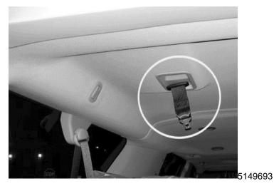
1. Remove the middle third row seatbelt buckle from the headliner seatbelt bezel.
