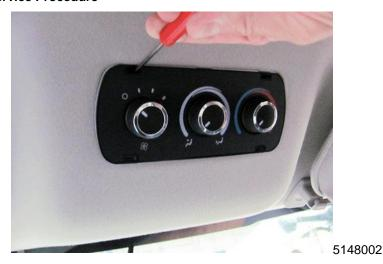
TIP: Use a small flat blade screwdriver to release the attachment tabs on the HVAC control.
