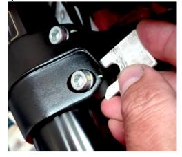
Take the new fork leg making sure that it is marked with the green marking near the screw hole of the lower fork leg:
