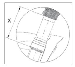
Loosen the screws of the upper triple clamp and of the lower triple clamp and remove the fork leg; to prevent damage to the components, we recommend using a plastic wedge to separate the parts slightly:
