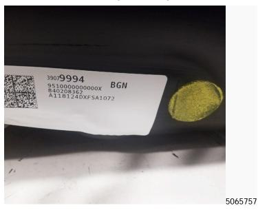
Inspect the fuel tank near the label (facing the rear of the vehicle) for the presence of a large yellow dot. If a dot is found, no further action is required, close the field action. If not, proceed to step 3.
