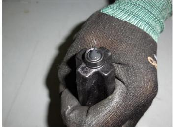
6. After applying glue, install phase cap into the cap hole on the HCA.
