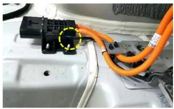
33. Remove the main wiring harness mounting clips.
