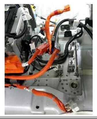
32. Remove the wiring mounting clips and ground bolt.
