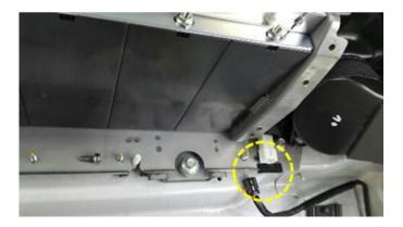
25. Remove the cooling duct mounting bolts and nuts.
