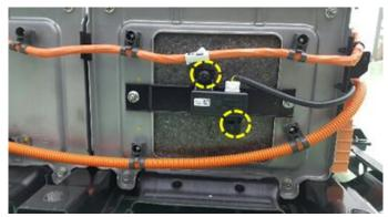
11. Remove the wiring mounting clips and disconnect the connector.
