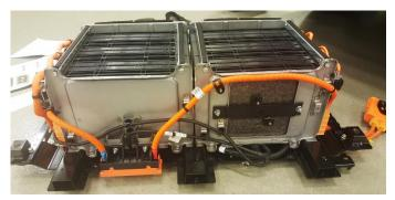
15. Reinstall the watertight cover to the Sub High Voltage Battery Pack.
