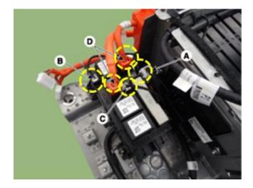
31. Remove the mounting bolts and remove the PRA (L).
