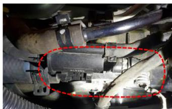
15. Remove the fuel pipe clamp bolt and bracket.
