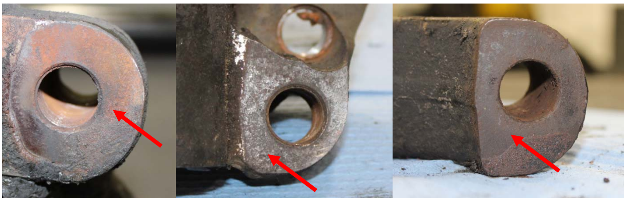
Figure 2 – Fretting Damage That May Look Like Rust from Water Intrusion at Loose Joint
