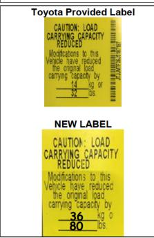
d. Calculate the NEW weight reduction rating by adding together the values from the Toyota provided label and all dealer installed accessory change weight values.
