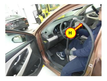
5. Remove the A-pillar trim (I) from both the LH and RH sides.
