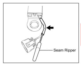
d. Using a seam ripper, carefully slice the black vinyl tube to remove it from the harness.
