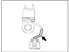
c. Unravel the vinyl tape from the outer end of the tube.
