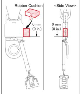
k. Peel the backing paper from the back of the **NEW** rubber cushion.
