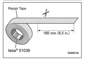
m. Cut a piece of the Tessa 51036 Abrasion Resistant tape to a length of approximately 160mm (6.3").
