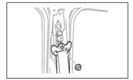
f. Install the shoulder anchor to the shoulder belt with the nut.
