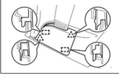
d. Install the 2 clips and 2 guides for the cover at the base of the Center Pillar Garnish.
