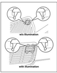
d. Attach the access cover on the step by engaging the claws.
