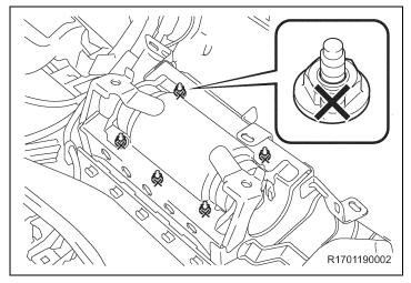
d) Mark the 5 self locking nuts to prevent reuse.
