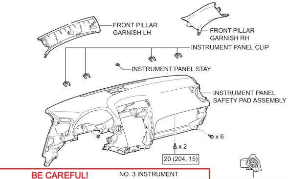
DO NOT pry from the outside with a moulding remover or the like.
