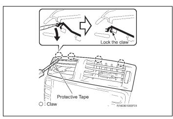
Removing the No. 3 air register
