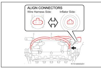
h) Connect the connector and the secondary lock.
