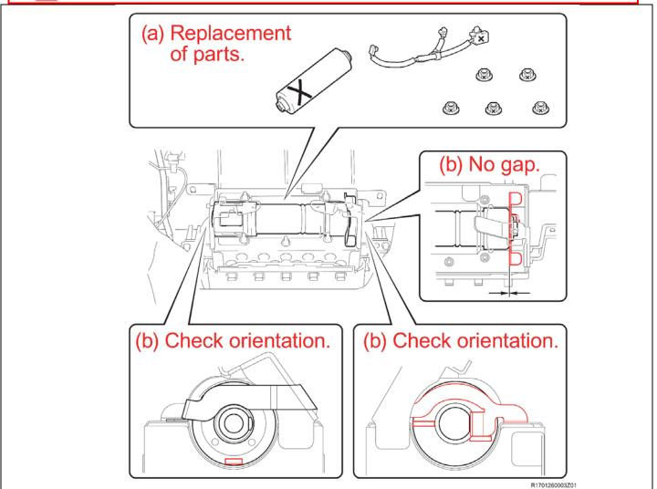
f) Tighten the 5 nuts evenly in several increments in the sequence shown. Use a socket driver or torque wrench to tighten the nuts.
