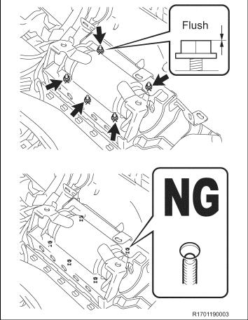
g) Loosen the 5 nuts until each nut is flush with the top of the stud as shown.
