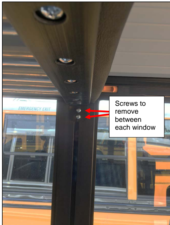
Figure 9: Removing the screws on rack at windows
