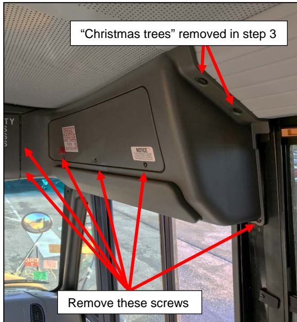
Figure 3: Entrance Door Cover & Screw Locations
