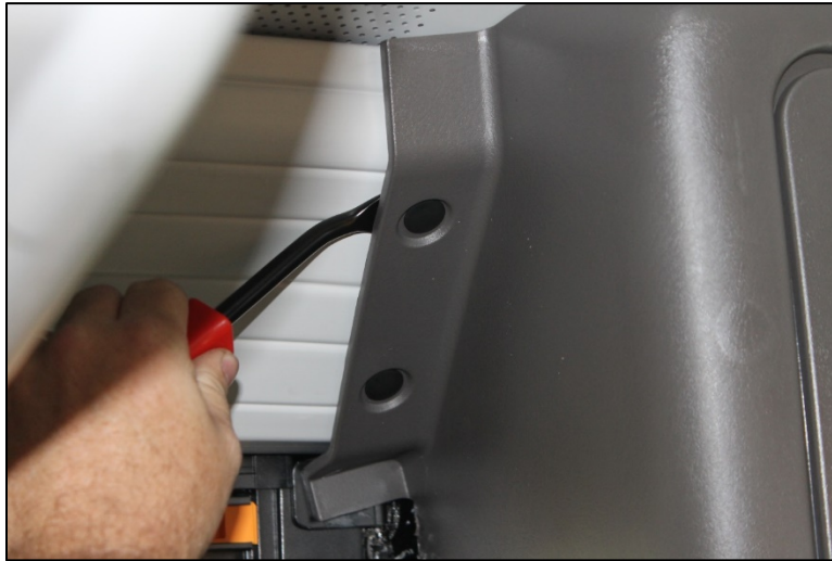
Figure 2: Removing "Christmas Trees" (Driver's Side Shown)
