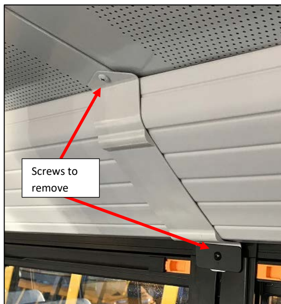
Figure 1: Header Cover Screw Location
