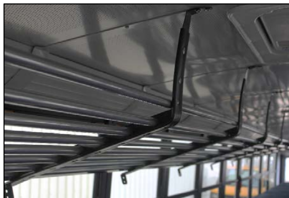
Figure 10: Luggage Rack Shown with Sidewall Screws Removed
