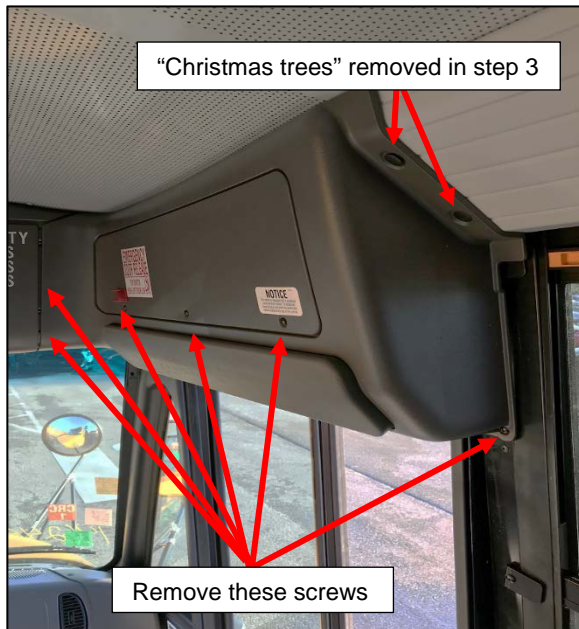
Figure 3: Entrance Door Cover & Screw Locations
