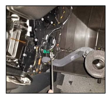
Remove glove compartment and inspect Auxiliary Heater Element -Z35- connector.
