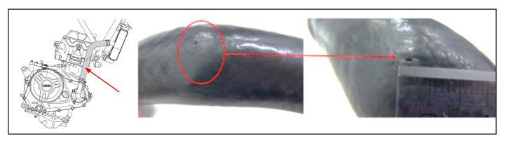
To correct this defect, Yamaha is initiating a Factory Modification Campaign. Affected units must have radiator Hose 3 replaced with a new one that was manufactured correctly.
