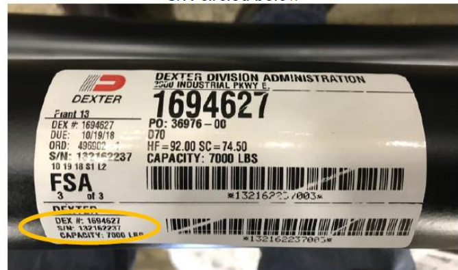
Serial Number (S/N) found on center of axle beam, S/N circled below
