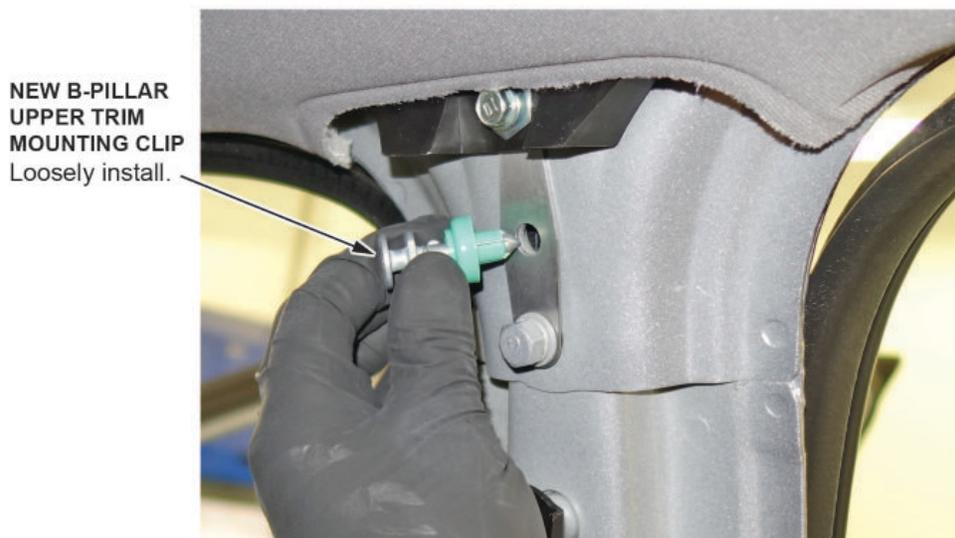
9.7. With the clip in the hole, torque the two bolts to the following specifications:
