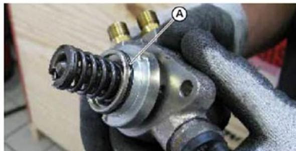
59. Install the pump and fasten them with the supplied screws (B). Alternate to each fasteners 2 turns of screws making the pumps perfectly adhere to their lodge.
