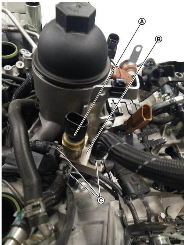
64. Install the feed rubber hoses (A,B,C). fasten the lines with the supplied clamps (D).
