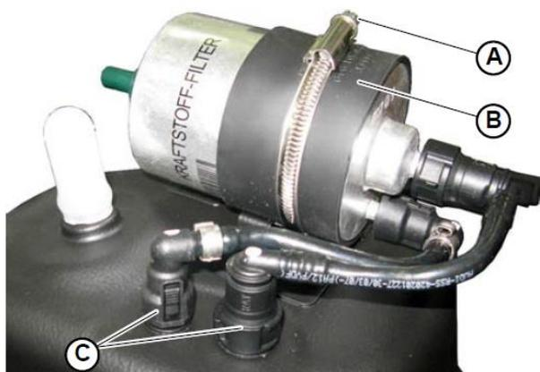
**Assembly of fuel feeding lines and high pressure pumps.**
