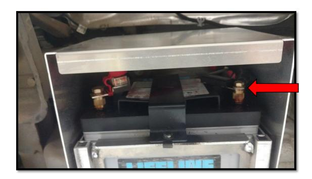
Step 5: Disengage the red rubber cap and, using the 13mm wrench, remove the containment nut on the positive fuse. Remove lock washer, flat washer and positive cable from the fuse side stud.
