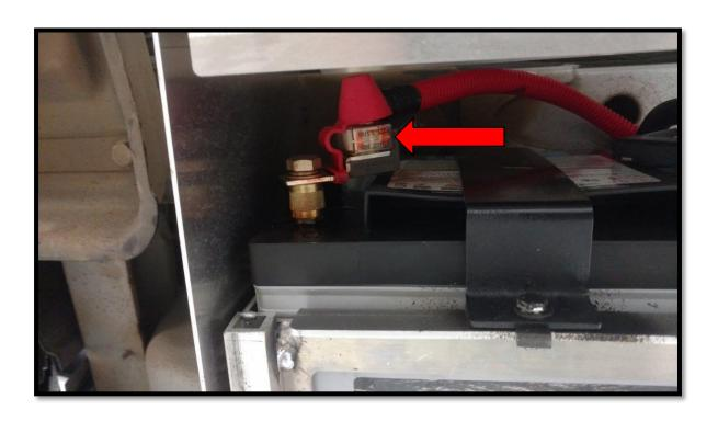
**Step 6:** Reconnect both coach battery ground cables. Torque to 70 in-lbs.
