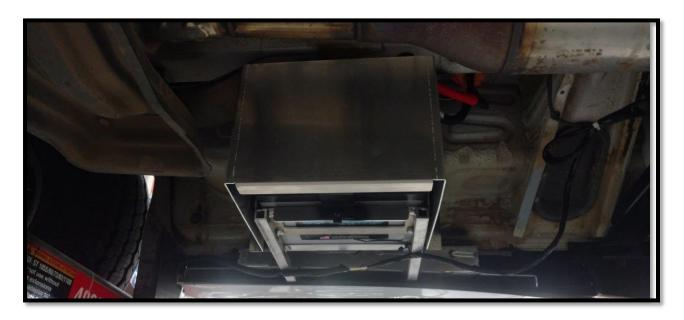
Using the 13mm wrench or socket, remove both battery negative cables and secure away from any ground point.
