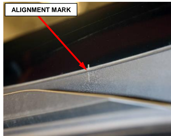
Figure 18 – Cowl Trim Alignment Mark in Middle of Windshield
