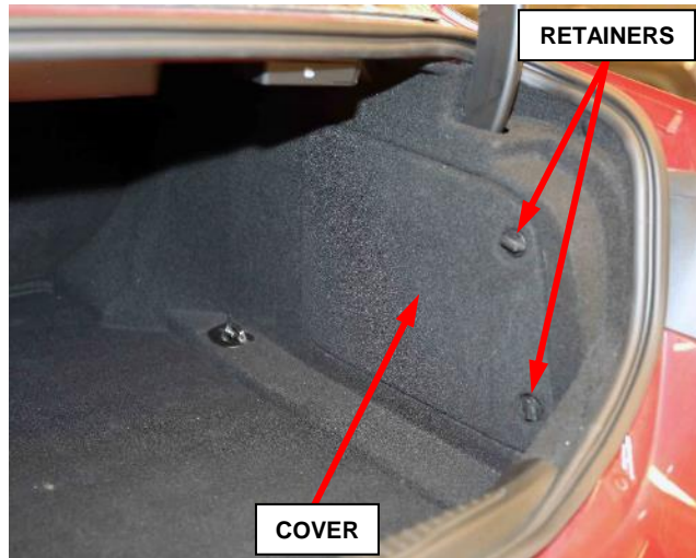
Figure 21 – Battery Access Cover
