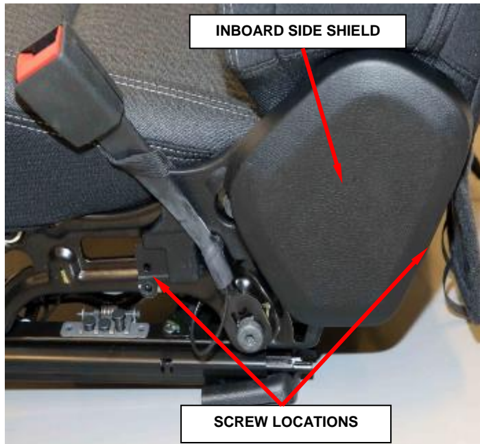
Figure 7 – Inboard Side Shield
