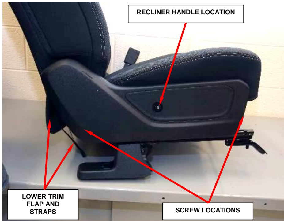
Figure 5 – Outboard Side Shield
