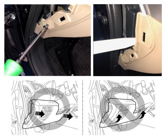
**REMINDER:** Before proceeding to **Step 6** below, it cannot be stressed enough for Technicians to **TAKE THEIR TIME** when removing and reinstalling the combination meter. The photos below illustrate what can happen to the meter assembly when not performing these steps **CAREFULLY**. These 3 examples all show damage caused by outside influence which is not a matter for warranty.
