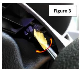
• Once the bezel is loose, disconnect the trip reset button harness connector and put the piece aside. On Push Start models, LEAVE THE START SWITCH CONNECTED and just flip the bezel over toward the radio. Cover the bezel with a clean shop cloth to make sure does not scratch the audio unit face or any surrounding trim.
