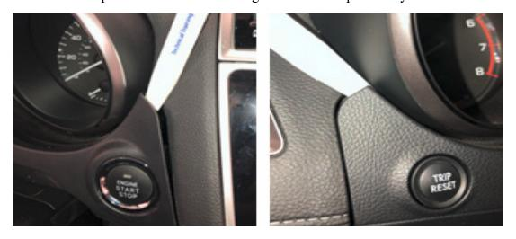
Release the lower claws on both ends of the bezel using a trim clip removal tool as shown.
