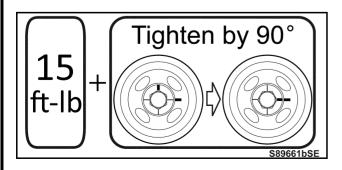
b) The crankshaft pulley must be tightened properly.
