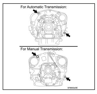
b) Reinstall the 2 transmission coupling bolts.
