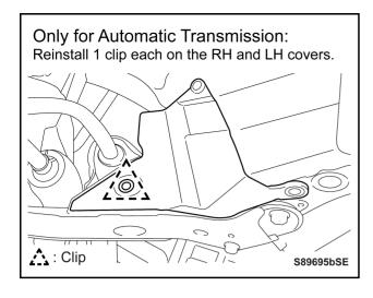
d) Reinstall 1 clip each on the left and right engine under covers.
