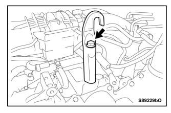
8. REMOVE ENGINE SLING DEVICE AND ENGINE HANGER
