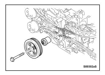
i) Temporarily install the spacer, the crankshaft pulley and the bolt.
