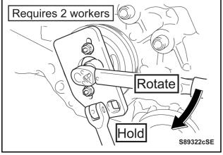
f) While another worker holds the crankshaft pulley in place using SST, install the bolt.
