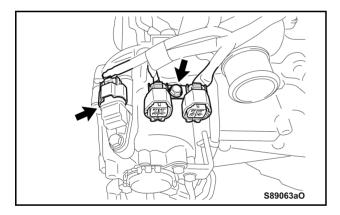
e) Reinstall the harness clamp bracket with the bolt. **Specified torque:**
