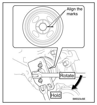
g) Draw a reference line on the crankshaft pulley set bolt, with a marker, according to the line engraved around the crankshaft pulley set bolt head (Mark the bolt).
