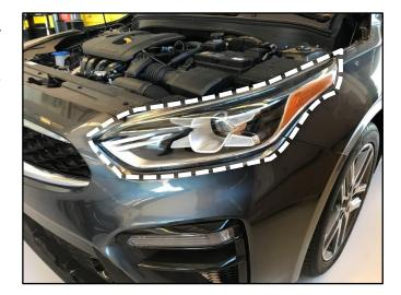
Verify proper operation and vertical aiming of headlamps and perform vertical adjustments using the banner, if necessary.
