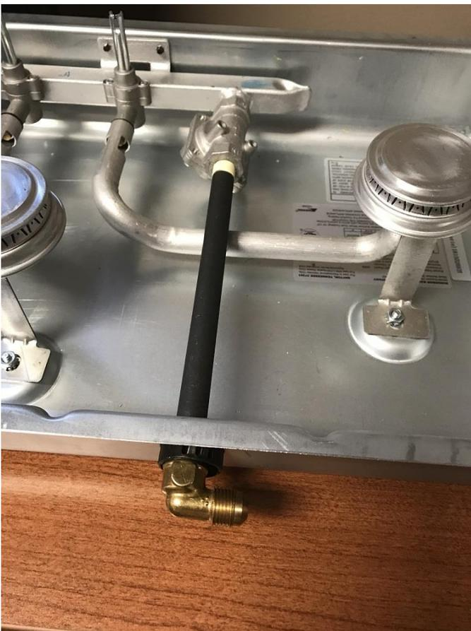
Note: in order to install the new pipe section, the 90 degree elbow can be fed through the grommet at the back of the burner box, or for easier installation, the entire 2 burner cooktop can be removed from the pullout tray by removing the screws from the side flange. (Cooktop removed in this image for visual clarification. )
