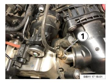
• Measure the temperature at the EGR cooler outlet pipe (1).
