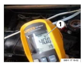
The temperature of the cooler needs to be below 50°C (1) before the probe of the digital video scope can be safely inserted to inspect the cooler.
