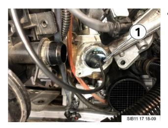
Insert the probe for the borescope and inspect the fins on the inlet side of the EGR cooler for any build up or contamination (1).
