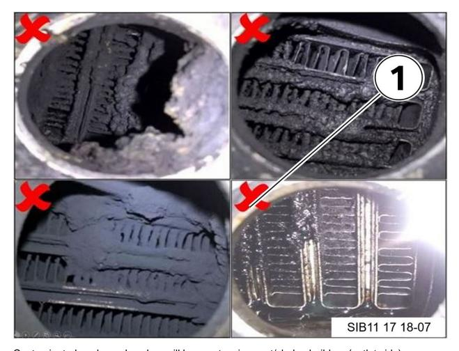
Contaminated or clogged coolers will have extensive soot/sludge build-up (outlet side).
