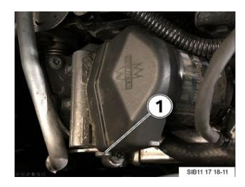
NOTE: (F15 is pictured) Remove the T30 screw (1) before removing EGR valve.
