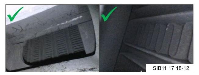
Clean or normal cooler with dry soot on fins (inlet side).
