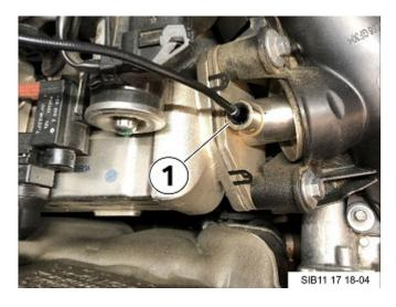
• Set the borescope to the 90° setting and install in the port temperature sensor (1).
