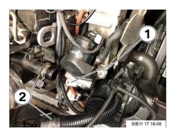
Loosen the tamperproof T30 screws (1) on the EGR valve and remove the valve from the EGR cooler. NOTE: The valve only needs to be removed from the cooler far enough to inspect the inside of the cooler. Do not disconnect the cooling lines from the EGR valve.
