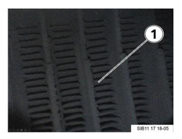
Inspect the fins on the EGR cooler for any build up or contamination. Black dry soot is a normal byproduct of the EGR system. An internally failed cooler will have a mix of soot and coolant which creates a moist "sludge" build-up. Attachment 2 to B11 17 18
