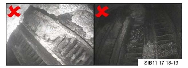
Contaminated or clogged coolers will have extensive build-up (inlet side).
