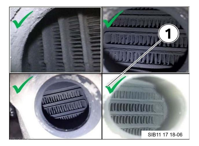
Clean or normal cooler with dry soot on fins (outlet side).
