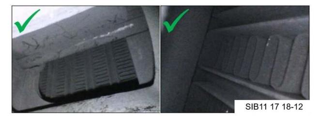
Clean or normal cooler with dry soot on fins (inlet side).
