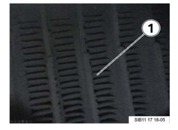
Inspect the fins on the EGR cooler for any build up or contamination. Black dry soot is a normal byproduct of the EGR system. An internally failed cooler will have a mix of soot and coolant which creates a moist "sludge" build-up.
