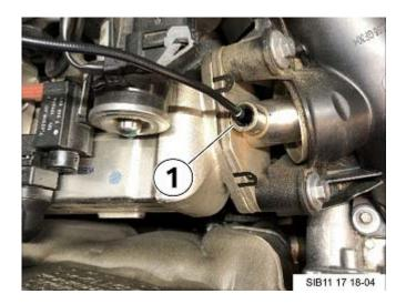
• Set the borescope to the 90° setting and install in the port temperature sensor (1).
