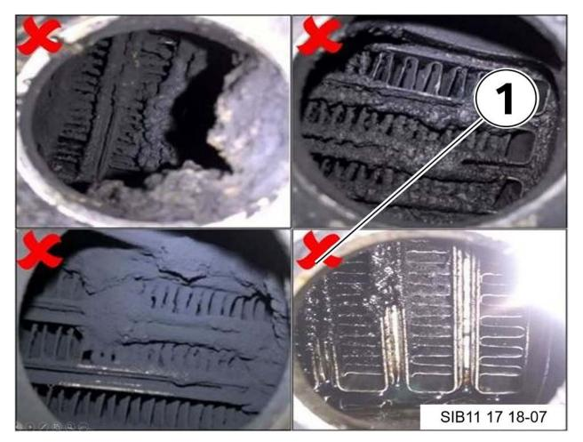
Contaminated or clogged coolers will have extensive soot/sludge build-up (outlet side).
