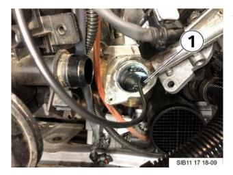
Insert the probe for the borescope and inspect the fins on the inlet side of the EGR cooler for any build up or contamination (1).
