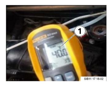
• The temperature of the cooler needs to be below 50°C (1) before the probe of the digital video scope can be safely inserted to inspect the cooler.
