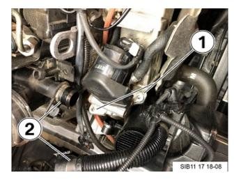
Loosen the tamperproof T30 screws (1) on the EGR valve and remove the valve from the EGR cooler. NOTE: The valve only needs to be removed from the cooler far enough to inspect the inside of the cooler. Do not disconnect the cooling lines from the EGR valve.
