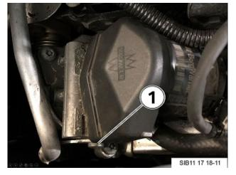
• **NOTE: (**F15 is pictured) Remove the T30 screw (1) before removing EGR valve.
